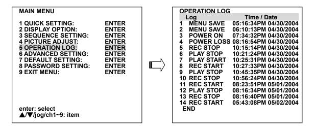
Note: The log keeps an operation history on a revolving basis because of its limit of 2000. When the log is full, the newly registered record of an operation will replace the existing records from the oldest one.
